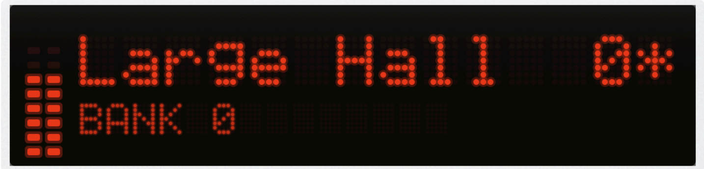
Register mode: label and slot number above, bank below. An empty or non-running slot shows the star.
