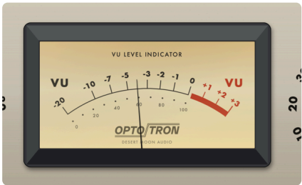
One meter, three jobs: gain reduction, or programme level at +4 or +10 calibration. The movement is a modelled moving-coil instrument, ballistics and all.
