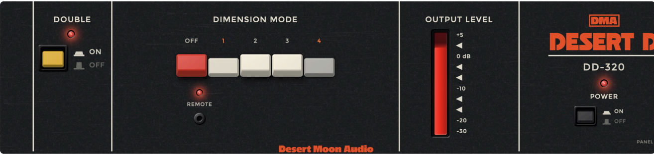
The front panel, running: DOUBLE in, mode 4 down, the meter at the box's nominal level, and the pilot lamp lit.
